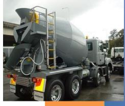
Full Refurbishment of Mixer Units - includes full assessment of job specifics :-Take off Bowl / Strip Down / Re-blasting / Chassis check and restructuring / Re-painting and realignment of mixer unit and frame.
